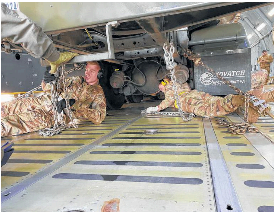
Reserve Citizen Airmen with the 26th and 74th Aerial Port Squadrons secure a fuel delivery truck to the floor of a C-5M Super Galaxy cargo aircraft during a training event Nov. 7 at Joint Base San Antonio-Lackland.
