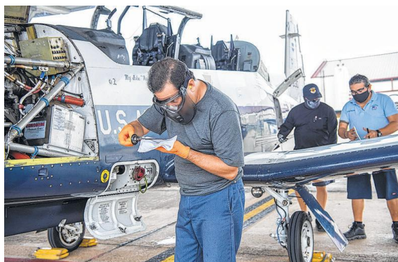
Greg Garcia, 12th Aircraft Maintenance Squadron, checks the oil of a T-6 Texan aircraft at Joint Base San Antonio-Randolph April 7.
