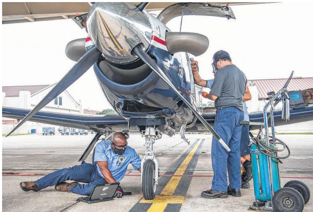
Shevon Vaciana, 12th Aircraft Maintenance Squadron, conducts routine maintenance by inspecting the front tire of a T-6 Texan aircraft at Joint Base San Antonio-Randolph April 7.
