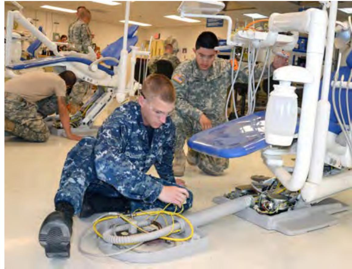
Petty Officer 2nd Class Brandon Richardson (left) and Pfc. Miguel Labra inspect the air supply on a dental treatment unit in the Dental and Sterilizer Equipment course.
