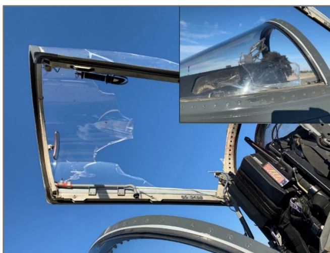
Figure 3-8. Bird strike damage on one of JBSA-RND's T-38s.
